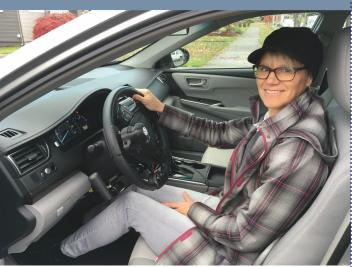
CHCS has a modified vehicle with SureGrip hand controls, a left foot gas accelerator and a passenger side brake. Behind the wheel evaluations will be conducted in this vehicle. Training will be provided on hand controls, if such adaptions are necessary for the client and his/her needs.
